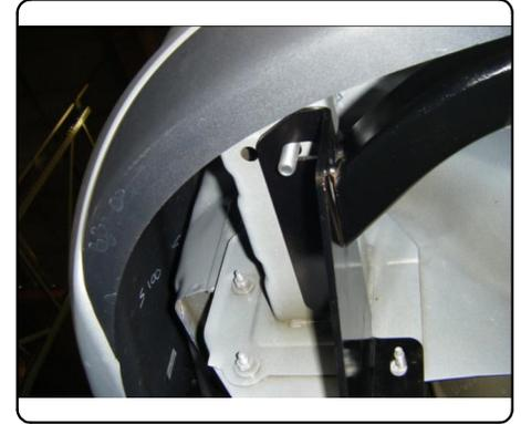
6. Secure all bolts with 7/16" flange nuts. Torque frontmost 7/16" hardware to 70 ft-lbs and rearwardmost 7/16" hardware to 50 lb-ft. Torque all 8mm hardware to 23 ft-lbs. Raise exhaust back into position.
