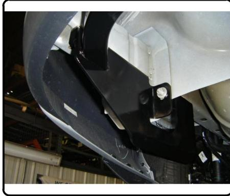
4. Fishwire 7/16-14 x 1 1/4" carriage bolt and SP7 spacer through upper and lower hole in the bumper bracket and out the rear-most hole in hitch, both sides.
