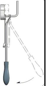
2. Remove existing 8mm nut from the inner most weld stud, both sides.
