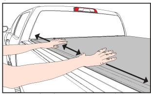
and both hook and loop engaged, use the palms of your hand to firmly push the loop strip into the hook track. Do this to both driver and passenger side up and down the entire length of the loop seams.
