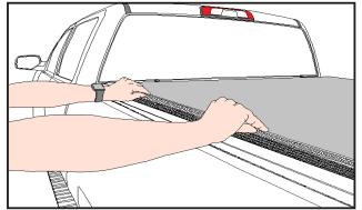
Engaging Hook and Loop, Step One: After rolling the cover Engaging Hook and Loop, Step Two: With the cover closed closed, grab the fabric loop flap and evenly pull loop over the hook track engaging the loop to the hook track. Avoid pulling fabric flap straight up.
