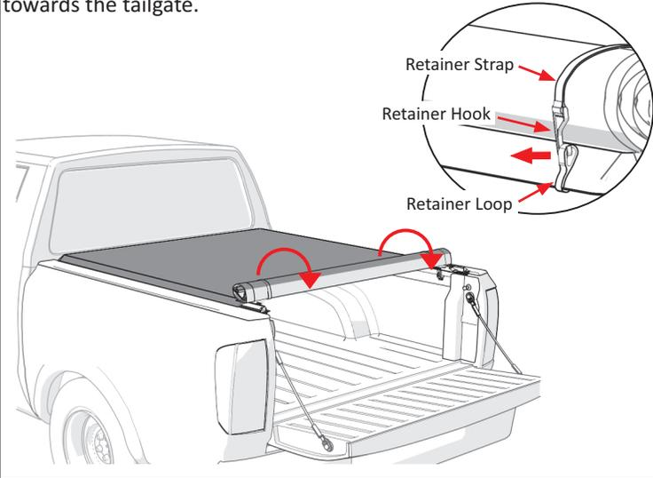
**13** Place the rear header into the header stops which are located on both side rails. Rotate the rear header downwards until you feel the cover latch in place.
