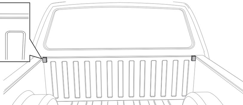
**4** Attach the end plug seals (G and H) to the front of the driver and passenger side rails (A and B).
