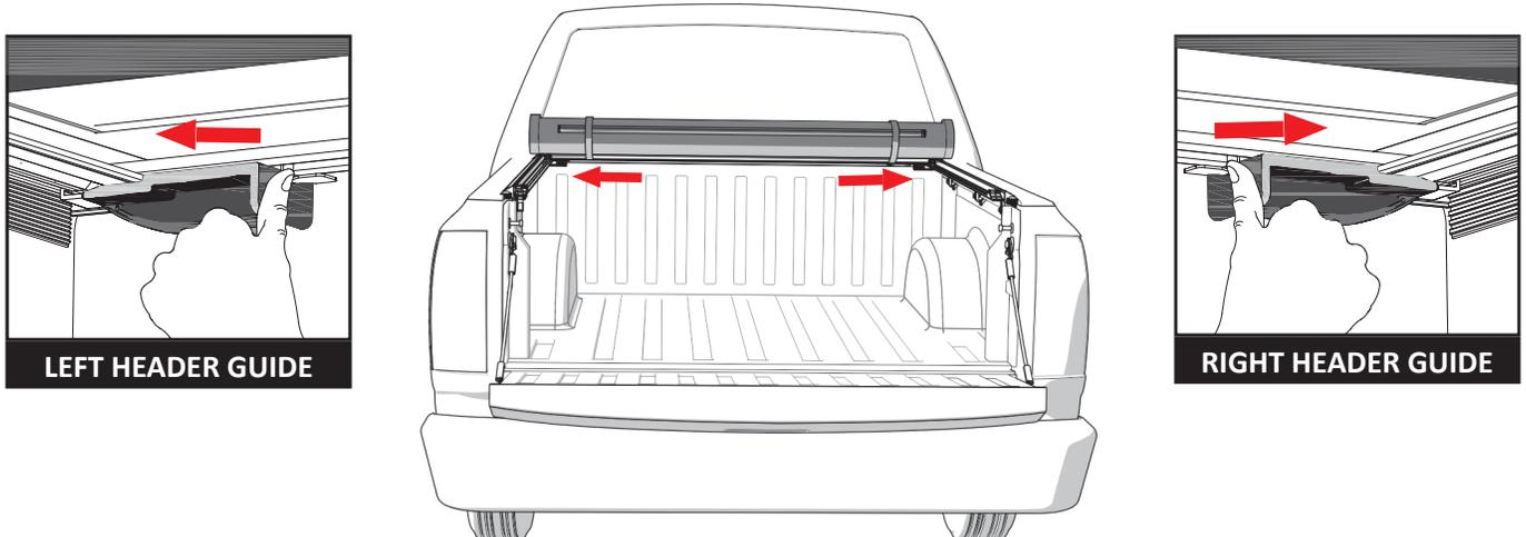
**12** To drive with the cover in the closed position, disengage the retainer hooks from the retainer loops and unroll the cover towards the tailgate.
