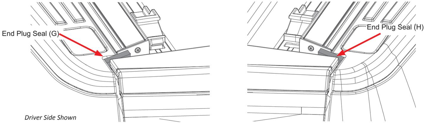
**NOTE:** If moisture does enter at the tailgate area then generally the moisture will run down the tailgate and out through the bottom of the tailgate and away from the truck.
