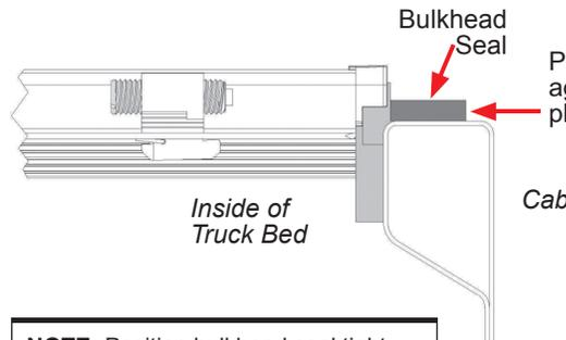
**NOTE:** Position bulkhead seal tight against rail endplug seal and bedcap.
