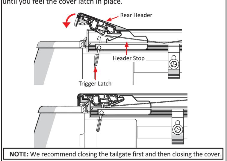
**14** A clicking sound will indicate a correctly installed cover. Next secure the hook and loop fastener along the entire length of both side rails before driving the vehicle. Simply run your hands down both sides of the cover to achieve this. This will prevent wind from lifting the cover and causing possible damage. **You are ready to drive with the cover in the closed position.**
