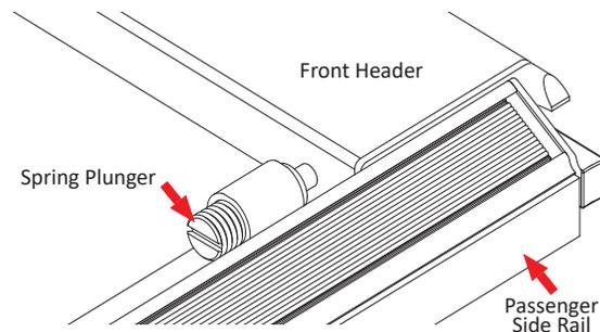
**NOTE:** Adjust tension in small increments. Slight adjustments will gain significant results.
