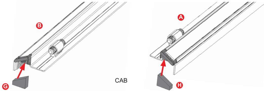
**5** Position the driver side rail (A) to the inside of the truck's bed rail. Adjust the rail vertically so that the seal is flush with the truck bed caps. The front edge of the rails will be 3/8" back from the bulkhead.
