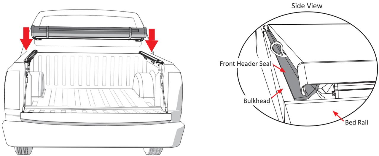
**11** To connect the cover assembly (C) to the side rails (A & B), slide the right and left header guides into the locked position. A clicking sound will indicate a secure attachment.
