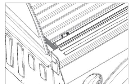
**9** Many truck tailgates, when closed, have corner gaps that allow moisture to enter the truck bed. Apply the end plug seals (G and H) to the side rail end plugs and truck bed corners to block moisture from entering the truck bed at the tailgate.
