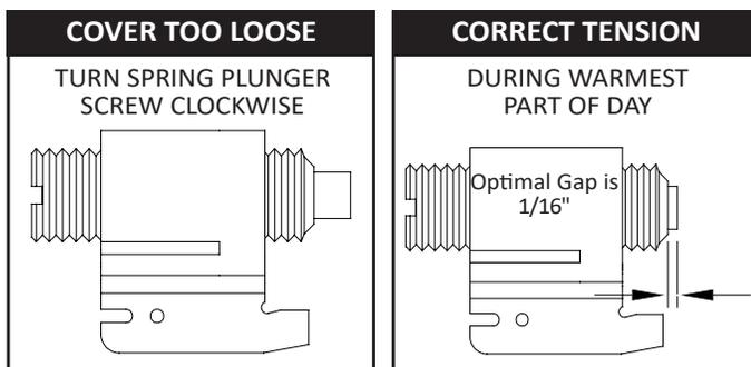
**NOTE:** Adjust tension in small increments. Slight adjustments will gain significant results.
