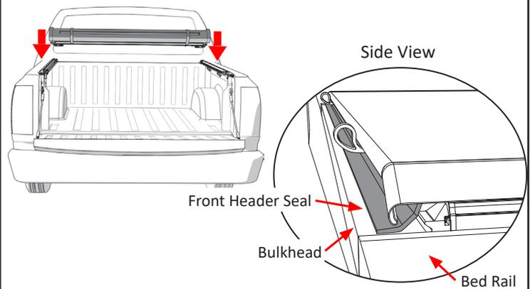
**10** To connect the cover assembly (C) to the side rails (A & B) follow these steps: Slide the right and left header guides into the locked position: Ensure that the header guides are aligned properly with the side rails.
