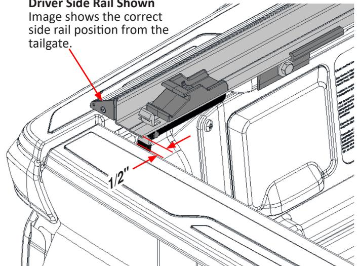
**8** The sets screws (I) can now be tightened into to the bottom side of the rail as shown below. Use the Allen hex wrench that has been supplied in the hardware bag to complete this step. Do this for each bracket.
