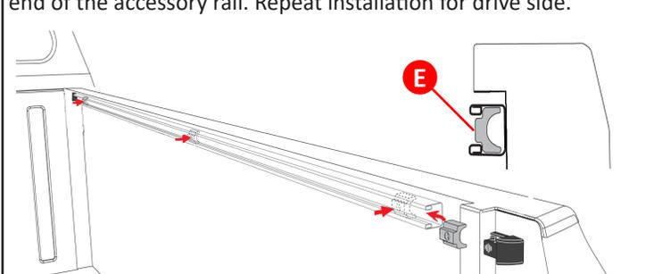
**6 Install set screws (I) to rail brackets (H):** Ensure you have the set screws (I), rail brackets (H), and Allen hex wrench required for installation.
