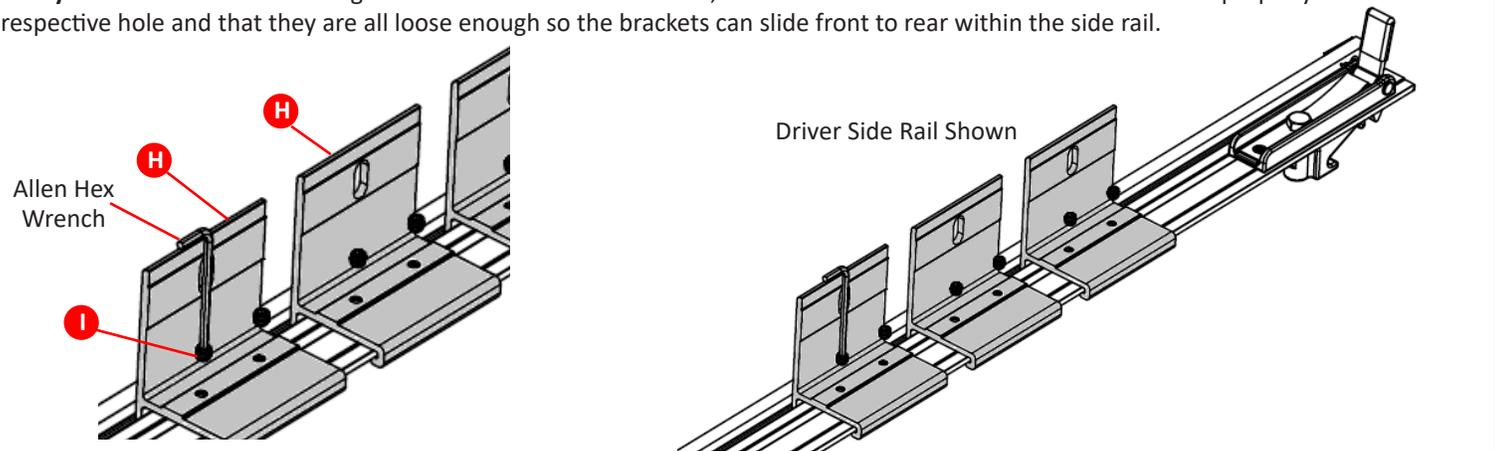
**7 Place assembled rails on bed caps:** Start by placing the assembled rails on top of the bed caps of the truck, ensuring that the fin seal is positioned on top. The fin seal helps to provide a secure fit and prevent water or debris from entering the truck bed.
