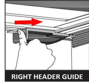
**11** Disengage the retainer hooks from the retainer loops: Locate the retainer hooks that secure the cover in place when closed. Disengage these hooks from the retainer loops by releasing them.
