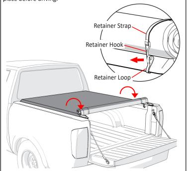
To latch and secure the cover properly, follow these steps: Place the rear header into the header stops: Locate the header stops on both side rails. These stops are designed to hold the rear header in place. Ensure that the rear header is positioned correctly within these stops.
