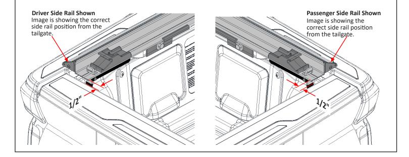
Positioning the side rails (A) and (B) from the bed caps at the tailgate end of the truck bed: At this point, the side rails should already be spaced correctly fore and aft (lengthwise), focusing now on the side-to-side spacing at the tailgate end.
