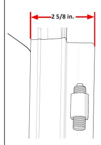
Space the driver and passenger side rails 2-5/8 inches from each bed cap at the cab end. While holding rail at 2-5/8 inches apply pressure downward on rail and tighten both bolts in each front bracket.
