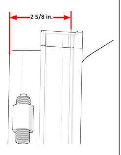
Place the cover (C) on the side rails towards the front of the truck bed (near the cab). The front header seal is designed to help shed water and should be sitting on top of the bulkhead.
