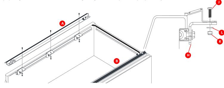
Position assembled side rails from the closed tailgate: With the truck's tailgate closed, position the end of each rail approximately 1/2" away from the rear corner of the truck bed. This positioning helps ensure proper alignment of the rail system and allows for clearance when opening and closing the tailgate.
