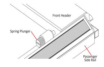
NOTE: Adjust tension in small increments. Slight adjustments will gain significant results.
