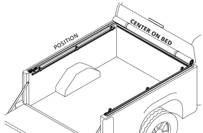
**10 Positioning of clamps at the cab:** The front clamps will use the inner groove to properly position the side rails at the front of the truck bed.
