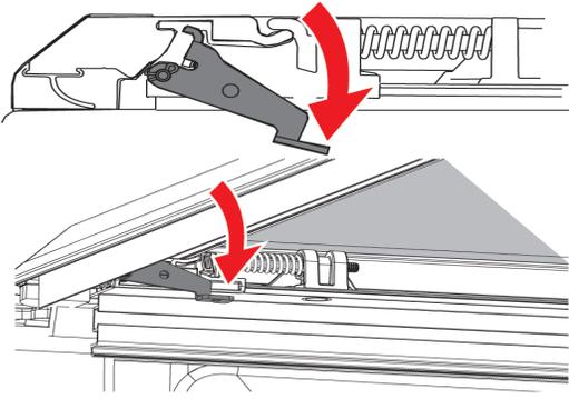
With the tailgate open, press down-ward on one side latch to disengage.
