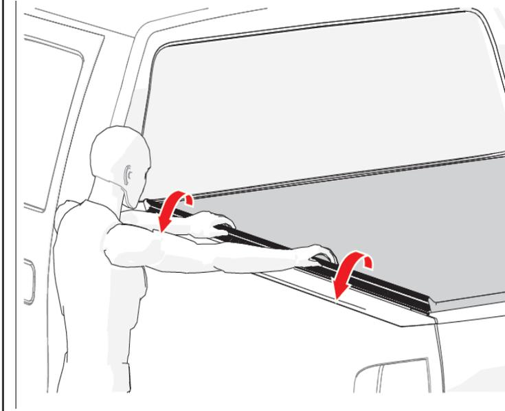
**21** Engaging the hook and loop: With both sides of the hook and loop engaged, use the palms of your hand to firmly push the loop strip into the hook track. Do this to both driver and passenger sides. **You are ready to drive with the cover in the closed position.**
