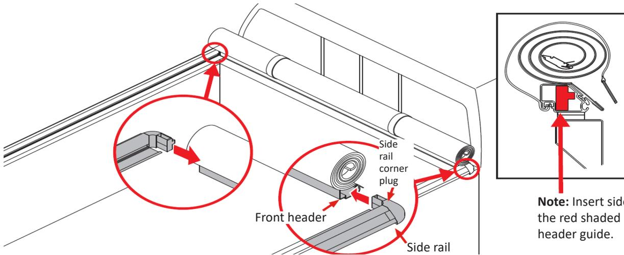
**Note:** Insert side rail into the red shaded area of header guide.
