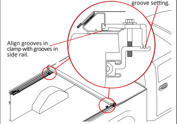
**12 Unroll the cover assembly (C) towards the tailgate.** Check that the side rails are centered on the truck bed. Note: that the spacing between the tailgate header and the side rails is 1/8" or 3.2 mm per side.
