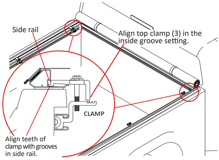
**11 Positioning middle clamps:** The middle clamps will use the middle groove to properly space the side rails in the middle of the bed.
