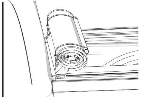
Roll up the cover. Do not disengage the hook and loop fasteners before rolling the cover. **Always secure the cover at the front with both retainer straps.**
