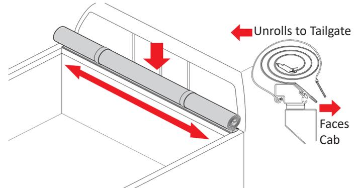
**8 To place the side rails:** Place the side rails (A & B) onto the truck bed rails and insert the side rail corner plugs into the front header, take care so the rails do not fall off of the truck and scratch paint.
