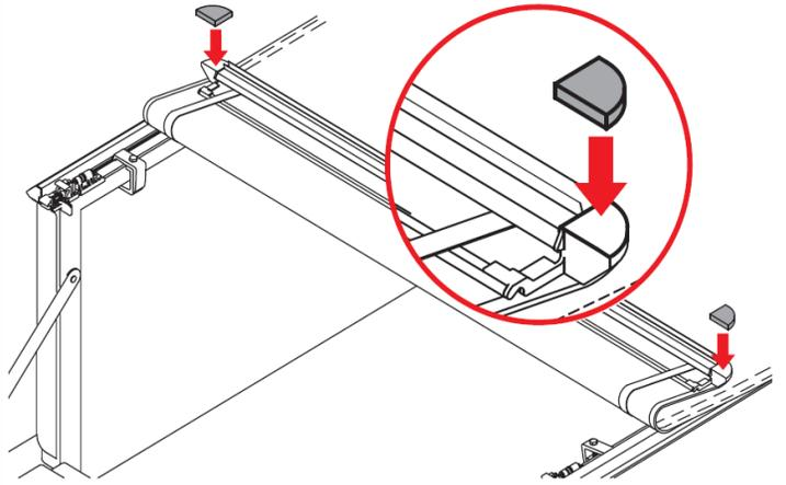
**18** Closing and latching down the rear header: With the tailgate open and the cover unrolled, hook the tailgate header into the header stops on both sides of the truck. Push the tailgate header down until the latches on both sides engage with the tailgate header. A clicking sound will indicate a secure attachment.
