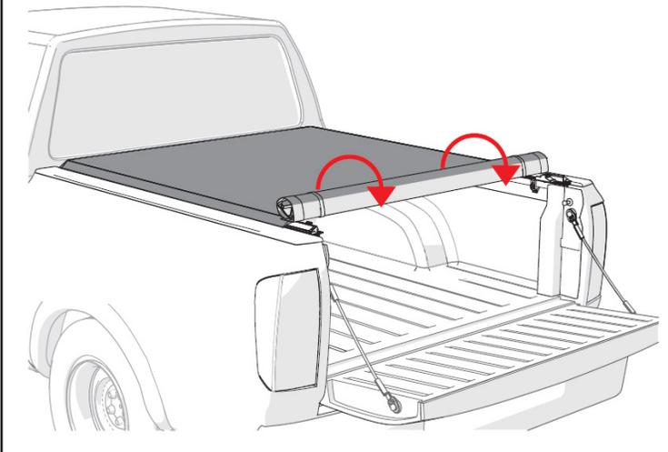
**17** Fold back the cover (C) at the tailgate, remove the adhesive backing and install tailgate corner seals (G), as shown.
