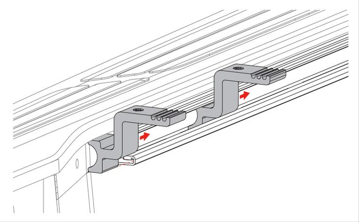
**6 Front corner end plug weather seal installation:** Peel off the cab corner seals (F) from the adhesive backing. Affix the cab corner seals (F) onto both cab end corner plugs located on the driver and passenger side rails (A & B).
