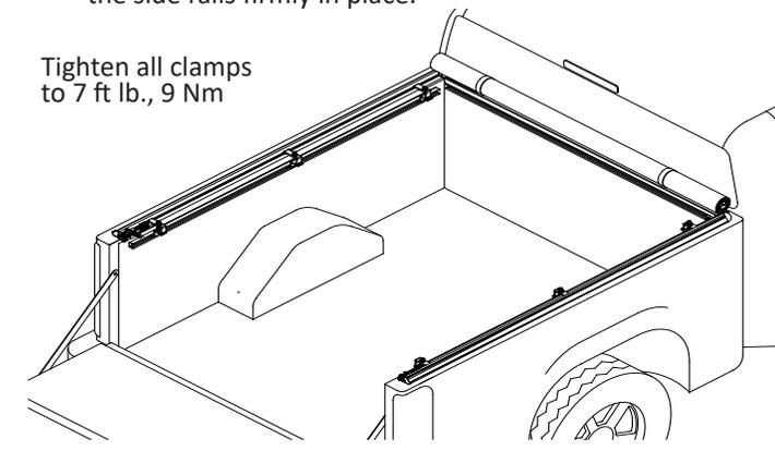
**15 Reinstall any tie-down cleats and the end cap on both sides of the truck bed.** Note: The tie-down cleats do not need to be inserted from the end of the cargo rails. They can be inserted at any location in the cargo rail. Review your trucks owners manual.
