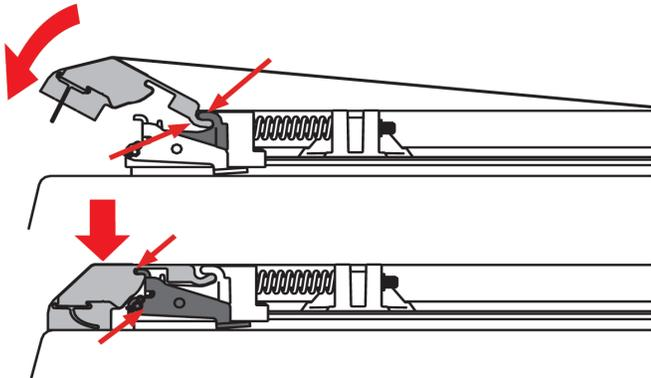
**19** Closing and latching down the rear header: Make sure the cover (C) latches on both sides of the truck. The latches will provide an audible click.
