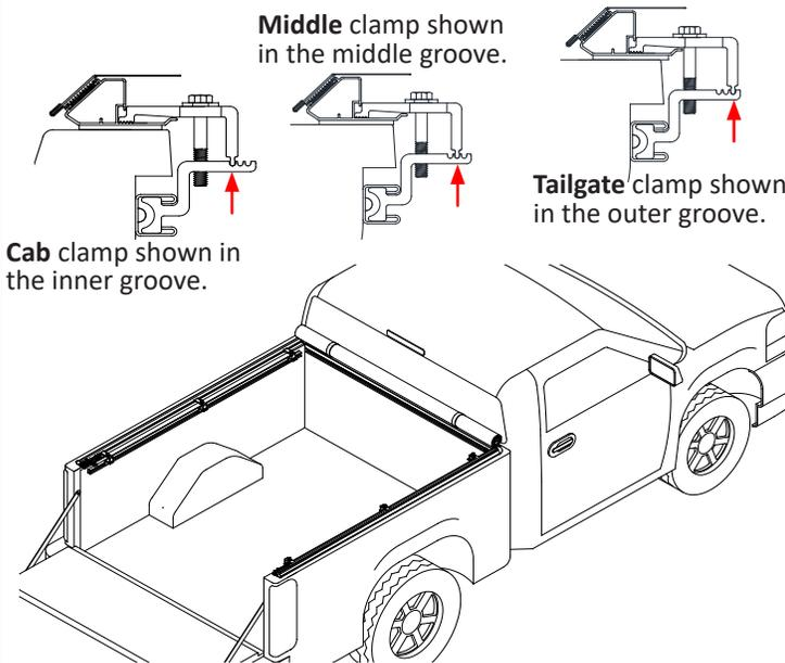
**9 Reassemble and space the clamps evenly:** Once assembled, evenly space each clamp along the bed rail of the truck.
