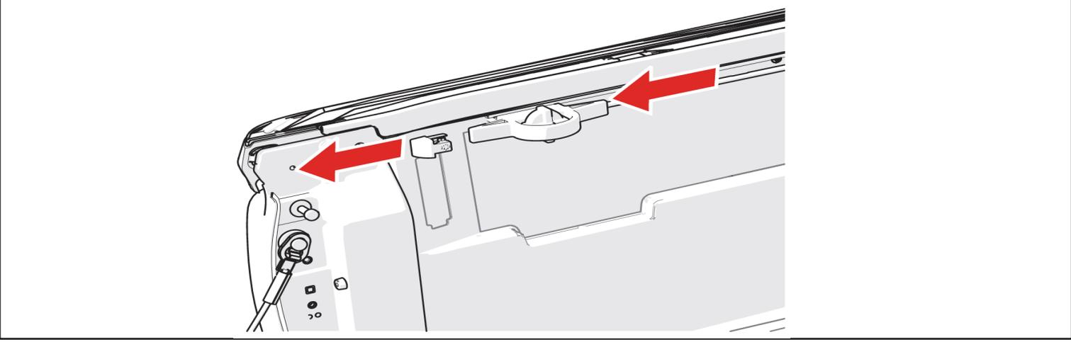
Disassemble clamps (E) as shown. Take care not to misplace clamp hardware.
