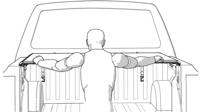
**NOTE: BOTH LATCHES MUST BE FULLY ENGAGED!**
