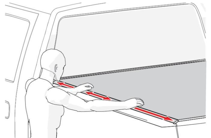
**HOOK AND LOOP MUST ALWAYS BE ADJUSTED AFTER ROLLING COVER CLOSED!**
