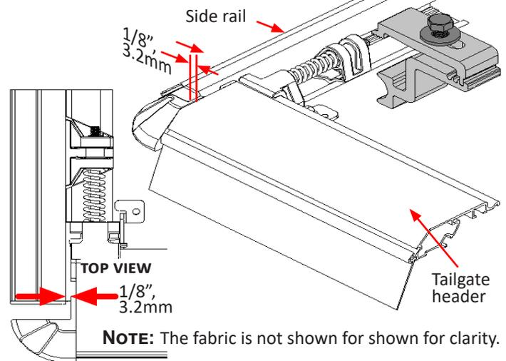
**13 Positioning of clamps:** The clamps positioned near the tailgate will use the outer groove.
