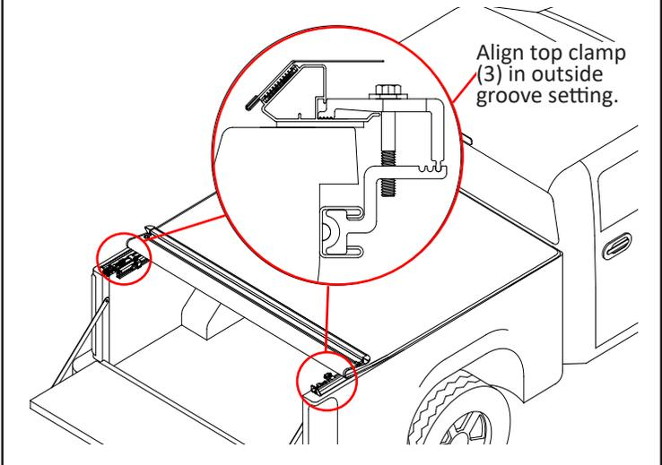
**14 Secure the clamps:** Roll the cover back to the front. After positioning the clamps correctly and connecting them to the side rails, securely tighten the clamps in position. Ensure that the clamps are tightened sufficiently to hold the side rails firmly in place.
