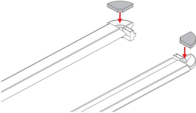
**7 Positioning the cover assembly (C) over the front bulkhead:** Position the cover assembly (C) near the truck's bulkhead, adjacent to the cab. Ensure that the cover assembly is oriented as depicted and is parallel to the bulkhead.
