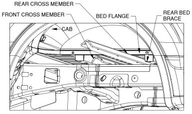
Figure B2: View of driver side wheel well.
