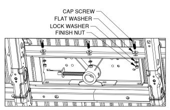
Figure B4: View under bed looking up at center section.
