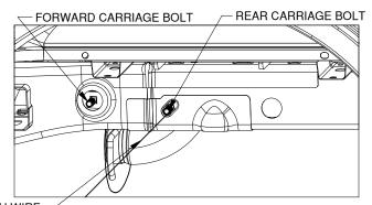
FISH WIRE — Figure C2: View of driver side wheel well.
