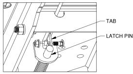
Figure E2: Handle Installation
