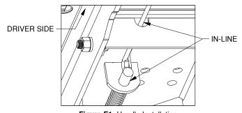
Figure E1: Handle Installation
