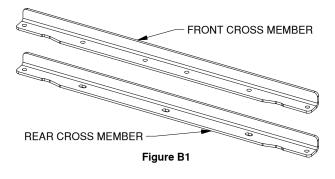
**NOTICE:** The gap between the bed flange and the frame may be narrower on some trucks than others. Most trucks have more clearance closer to the rear bed brace. If the cross members cannot be placed without damaging the paint, a small notch can be put in the bed flange for added clearance.
