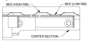
Figure F1: Cutaway view of bed and center section.
