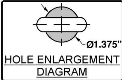
4. Reverse fishwire 1/2" x 1 1/2" carriage bolts and CM-SP17 spacers into holes enlarged in Step 3. Install 1/2" x 1 3/4" carriage bolt and CM-SP4 spacer through top of vehicle tow loop.
