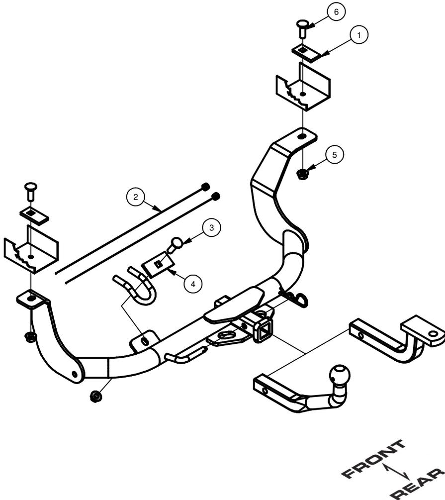
1. Lower exhaust by removing (2) exhaust isolators. Remove rubber plug from hole on driver side of vehicle.
