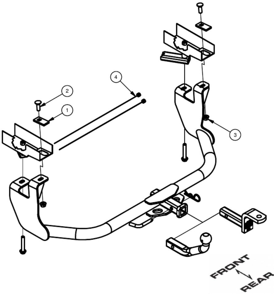
1. Remove existing bolt from driver and passenger side of vehicle. Retain bolt for hitch installation
