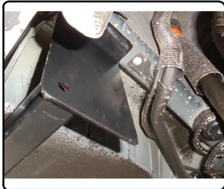
5. Install 1/2" carriage bolt with large square hole spacer through tow hook and support bar on hitch and fasten with 1/2" flange nut, as shown.
