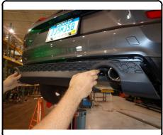
2. Fishwire (2) 1/2"carriage bolts and spacer blocks through driver side access hole in bumper beam.
