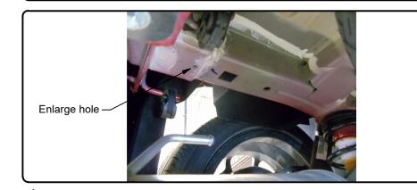
4. Raise hitch into position, taking care not to push carriage bolts back into frame and sandwiching hitch passenger side plate between frame rail and spare tire control box, if equipped. Install M8 hex bolts and 7/16" conical toothed washers into weldnuts in passenger side frame rail. Install flanged hex nuts onto carriage bolts in driver side frame rail. Torque all 7/16" fasteners to 59 lb.-ft.; Torque all M8 fasteners to 23 lb.-ft.
