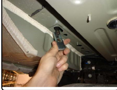
8. Raise hitch into position, being careful not to push bolts back into frame. Secure with 1/2" hex flange nuts. Torque all 1/2" hardware to 110 lb-ft.
