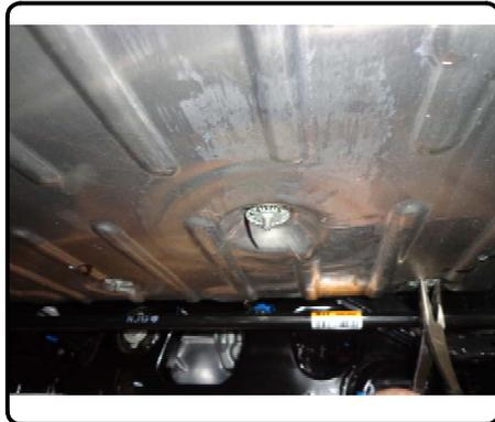
5. Mark heat shield as shown to trim for receiver tube clearance (6" wide) and to allow access to both frame rails. Reattach trimmed heat shield using (8) of the nuts removed in Step 4.
