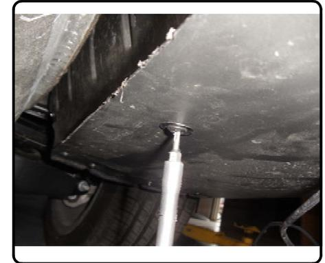
2. Gently pull inner fender material toward tire on each side and remove top bolt with 7mm socket. Pull off fascia completely and disconnect electrical connector from driver side.
