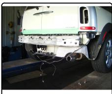
12. An access hole will need to be drilled through your bumper cover to allow access to the receiver tube. Mark your drill location by measuring down from the bumper cover lip 3-3/4" and center by using the dimple in the license plate cover. Using a 2-1/2" hole saw drill through the license plate holder and bumper cover. When drilling make sure not to drill through the sensor bracket or loose wiring. NOTE: Verify drill location prior to drilling!
