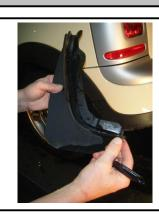
4. Slide one hand past the wheel well liner and fender flare, then push up on the (2) lower tabs that connect the fender flare to the bumper cover (Note: See the first photo in Step (5) for tab clarity). Using your other hand pry the rear fender flare away from the car until it pops free. Release side marker bulb from fender flare.
