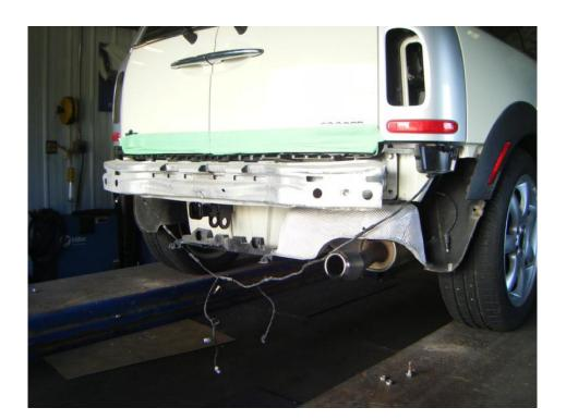
12. An access hole will need to be drilled through your bumper cover to allow access to the receiver tube. Mark your drill location by measuring down from the bumper cover lip 3-3/4" and center by using the dimple in the license plate cover. Using a 2-1/2" hole saw drill through the license plate holder and bumper cover. When drilling make sure not to drill through the sensor bracket or loose wiring.
