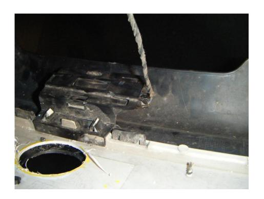
14. Align bumper cover and pull back on the fender flare. Push bumper lock tabs in place until they snap. Re-attach side marker bulbs to fender flare. Reinstall all (8) fasteners removed previously and snap fender flare back into place.
