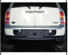
15. The first photo shows hitch fully installed when not in use. The second photo shows hitch ready for use with safety chains attached. **Note:** Trailer not shown.
