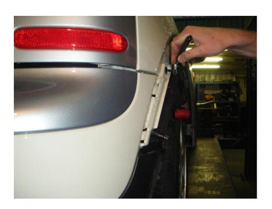
6. Using a phillips screwdriver, remove fastener 4 from the bottom of the bumper cover.
