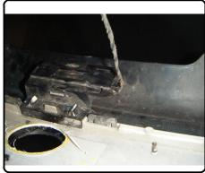
14. Align bumper cover and pull back on the fender flares. Push bumper lock tabs in place until they snap. Re-attach side marker bulbs to fender flares. Reinstall all (8) fasteners removed previously and snap fender flares back into place.
