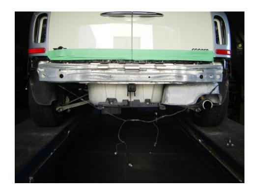
11. Secure hitch using (4) 8mm bolts and (4) 8mm nuts removed in Step (9). Torque all 8mm hardware to 24 ft-lbs.
