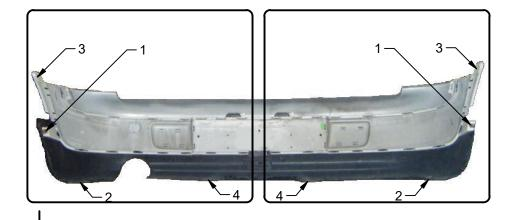
2. Using a phillips screwdriver remove fastener 1 from inside the rear wheel well. **Note:** If needed you may remove the rear wheels to access screws.
