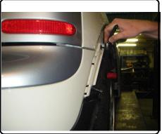
6. Using a phillips screwdriver, remove fastener 4 from the bottom of bumper cover.
