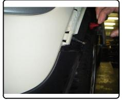
5. The first photo shows the lower fender flare tabs released. Using an offset phillips screw driver or wrench with a phillips driver bit remove hidden fastener 3 behind the fender flare.
