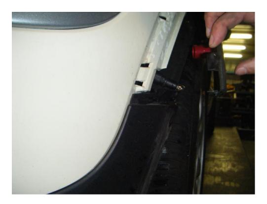
5. The first photo shows the lower fender flare tabs released. Using an offset phillips screwdriver or wrench with a phillips drive bit remove hidden fastener 3 behind the fender flare.
