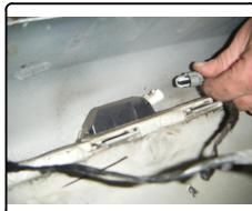
8. The first photo shows the bumper cover removed, exposing the aluminum bumper beam. Using a flat blade screwdriver remove the (7) wiring harness clips from the bumper beam.
