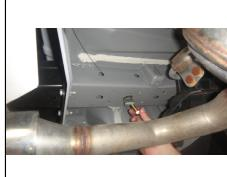
4. Raise hitch into position and pull the fishwires and carriage bolts through the side plates. **Note:** Feed the fishwires through the mouting holes while raising the hitch. Remove the fishwires from the carriage bolts and secure the hitch with 7/16" flange nuts.
