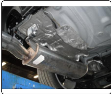
2) Remove the exhaust heat shield from the driver side and the plastic underbody panel on the passenger side. Keep fasteners for later re-installation.
