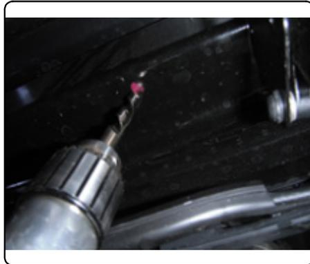
6. Fishwire 1/2" x 2" carriage bolts and CM-SP4 spacers through the access holes between the fascia and the back of the bumper beam and out the holes drilled in Step 5. Raise hitch into position and secure with 1/2" flange nuts.
