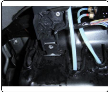
2. Remove the plastic underbody panel for trimming by removing (6) plastic retainer nuts with a 10mm socket.
