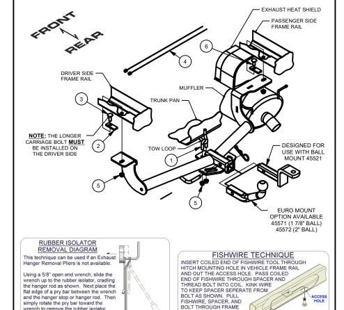
Note: On Front wheel drive models, the lower underbody panel may need to be trimmed as shown below to install the hitch. The exhaust heat shield will need to be bent approximately 3/4" to allow hitch to rest flat against the frame.
