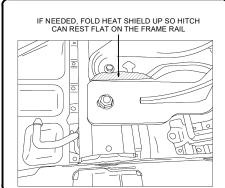
2. On the driver side, fishwire a 7/16-14 x 1 1/4" carriage bolt and SP2 spacer through an existing fore hole. On the passenger side, fishwire a 7/16-14 x 1" carriage bolt and SP2 spacer through an existing fore hole. Note: The longer carriage bolt must be installed on the driver side.
