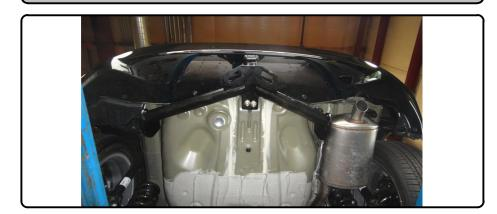
4. Secure hitch to the frame rails using 7/16" flange nuts.
