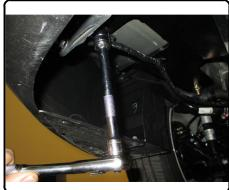
6. Torque all 7/16" hardware to 70 ft-lbs. Reconnect electrical harness through clearance hole on driver side frame rail.
