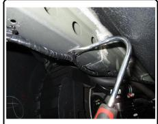
2. Enlarge access hole forward of tow loop on passenger side frame rail to allow 7/16" carriage bolts and CM-SP11 spacers to pass through.
