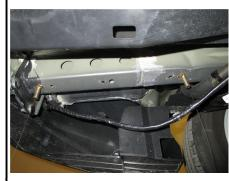
5. Raise hitch over exhaust into position and pull fishwires and carriage bolts through side plates. **Note:** Feed fishwires through mounting holes while raising hitch. Remove fishwires from carriage bolts and secure hitch with 7/16" flange nuts.
