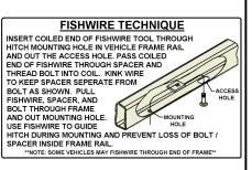
4. On driver side frame rail, fishwire two (2) 7/16" bolts and two (2) CM-SP11 spacers through holes on side of frame rail and out existing holes in bottom of frame, as shown. <u>Note:</u> Leave fishwires attached to prevent loss into frame rails.
