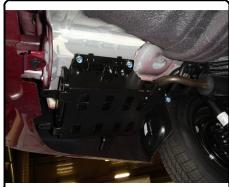
2. Rotate canister downward to provide access to the frame rail. Remove exposed (2) M10 screws using a 12mm socket. Save for reinstallation in Step 3.
