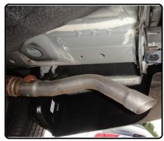
4. Place u-bolt into position in the vehicle recovery loop. Raise the hitch into position in between the last bracket removed in Step 1 and the driver side frame rail. Loosely secure with provided M8 bolts and conical tooth washers on the driver side. Secure remaining fasteners using 3/8" flange nuts.
