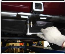
5. Tighten 3/8" bolts to 37 ft-lbs. Tighten M8 bolts to 23 ft-lbs. Repeat Step 1 in reverse order to reinstall components removed from the vehicle. If desired trim underbody panel as shown below using contours of the part as a guide.
