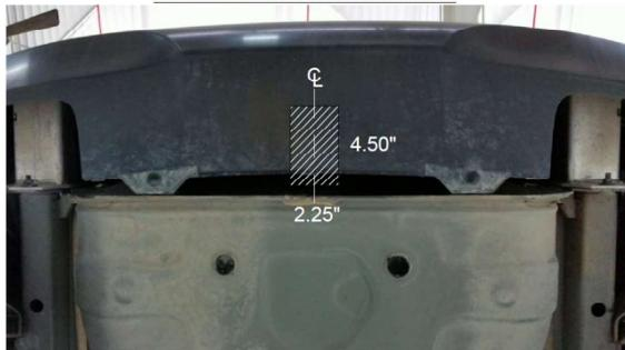
4. Raise hitch into position and loosely secure using existing vehicle hardware.
