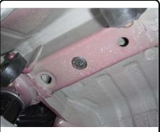
Fishwire 7/16" carriage bolts and CM-SP11 spacers into position first and reverse fishwire 1/2" carriage bolts and CM-SP6 spacers into position afterward. (enlarge access hole as necessary)
