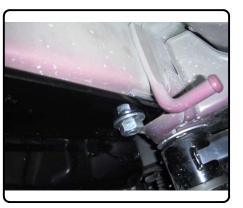
4) Torque all 7/16" fasteners to 59 lb-ft, and all 1/2" fasteners to 110 lb-ft.
