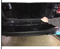
5. Remove (4) clips holding plastic bumper panel to bumper beam. Remove (2) nuts from each side using 18mm socket. Insert hitch between bumper beam and vehicle. Loosely secure existing hardware.
