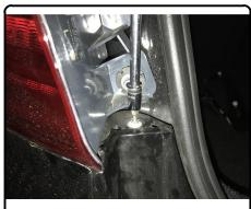
4. Remove (2) bolts using 10mm socket from each tail light. Carefully remove rear bumper fascia. <u>NOTE:</u> To ease fascia removal, begin from outside and work towards the center of the vehicle.
