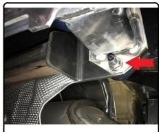
6. Trim underbody panel along slotted line. Torque all M12 hardware to 82.5 ft-lbs. Reinstall removed items following steps 1-5 in reverse order.
