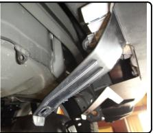
Raise hitch into position and install supplied fasteners as shown. Torque all 3/8" fasteners to 37 lb-ft and all 5/8" fasteners to 180 lb feet. Re-install remaining bumper fascia tabs to original positions.
