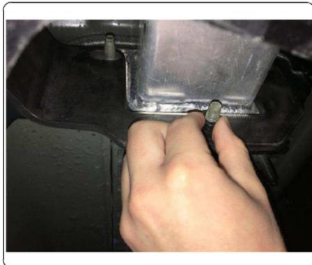
5. Use 15mm socket and torque all vehicle hardware to 45 ft-lbs. Reinstall hardware removed in step 1.
