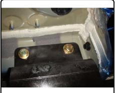
Reattach exhaust hanger and reinstall underbody panel removed in Step 1.
