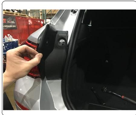
5. Remove (2) bolts from each tail light using 10mm socket. Carefully remove tail light from vehicle and unclip electrical harness.
