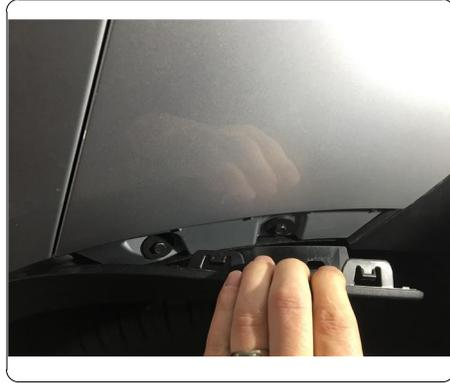
4. Open rear hatch to expose and remove plastic cover located inboard of each tail light, remove (1) fastener on each side flathead screwdriver.
