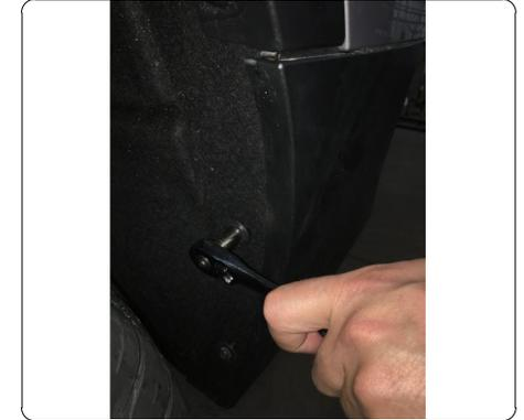
2. Remove (3) rivets along wheel well trim above each rear tire using a small punch and pry tool. **NOTE:** Replacement rivets are included.
