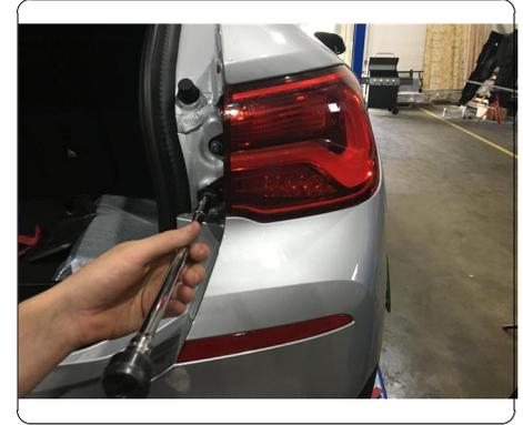
6. Remove rear fascia by locating and removing fastener behind tail light cover using 8mm socket and unclip rear fascia attachments.
