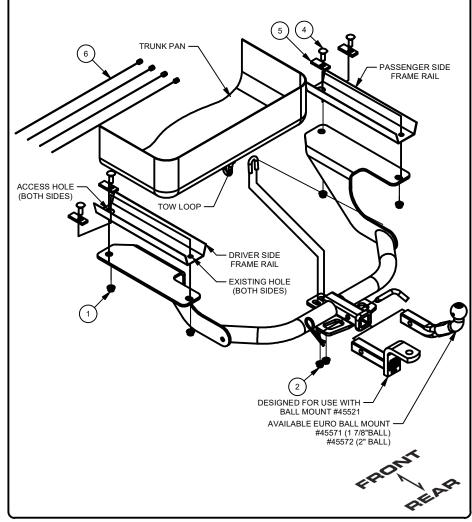
1. Lower exhaust by removing (4) rubber exhaust isolators See RUBBER ISOLATOR REMOVAL DIAGRAM below.
