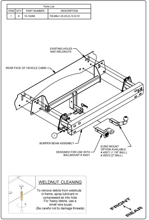
1. C-HR: Remove (14) push pin fasteners and (3) twist type fasteners attaching (2) underbody panels to the rear of the vehicle. Locate and remove the (6) fascia clips holding the lower bumper fascia to the rear bumper body panel. Corolla Hatchback: Remove the center portion of the rear bumper fascia by removing the lowest screw from each side of the rear of the bumper cover then push out the tabs on the back. Note: There are 2 wire harness mounting clips on the top that need to be removed.
