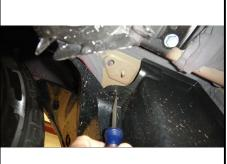
2. Using a 12mm socket, remove the (8) bolts attaching the bumper assembly to the rear face of the cabin. Lightly pull the lower fascia away to remove the bumper beam and return flange bolts to vehicle owner.
