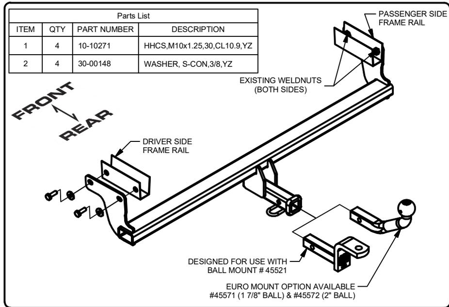
2. Locate and remove the wheel well push pins on each side of the vehicle. Lift hitch into position and secure to the vehicle using (4) M10 hex bolts and (4) 3/8" conical tooth washers. With the hitch in position, reconnect the electrical harness.
