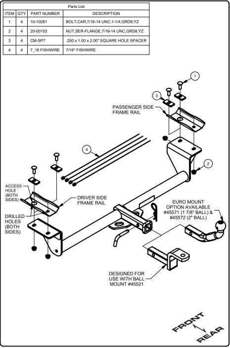
1. Raise hitch into position against the back of the frame rail. Using the hitch as a template, center the holes on the frame rail and use a paint pen to mark out the (4) hole locations.
