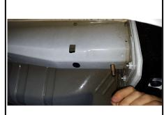
Using the forward-most holes that were enlarged in step 3, reverse fishwire (2) 7/16" carriage bolts and (2) CM-SP7 spacers into the frame. (See reverse fishwire diagram).
