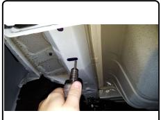
Using the forward-most holes that were enlarged in step 3, fishwire (2) 7/16" carriage bolts and (2) CM-SP7 spacers into the rear most holes. (See fishwire diagram).
