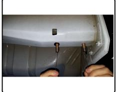
6. Raise hitch into position running the fishwires through the holes on the hitch. Remove fishwires and loosely fasten (4) 7/16" flange nuts.
