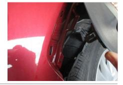
Carefully pull the trim away from the vehicle enough to remove the plastic push rivet at the top of the bumper cover on each side of the vehicle.
