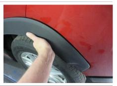
Reinstall the mudguards and taillights removed earlier.
