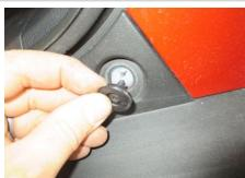
If present, remove the mudguards by removing the four screws securing each guard with a 10mm socket. Remove the two plastic push rivets located under the bumper cover near the muffler with a flathead screwdriver.
