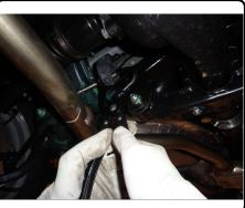
2. Remove (4) heat shield attachments with phillips head screwdiver or 10mm socket (both sides if equipped with dual exhaust). Remove three hole plugs from each side of frame to expose mounting holes. Return all removed items to customer.
