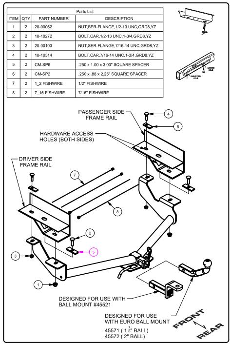
1. Reverse fishwire 7/16" carriage bolts and spacers to forward mounting holes in frame, fishwire 1/2" carriage bolts and spacers to rear mounting holes in frame though access holes. (BOTH SIDES)
