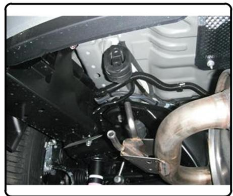
2. If present, remove the tow loop on the passenger side of the vehicle frame. Return tow loop and bolts to vehicle owner.
