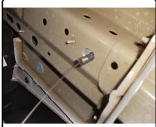
4. Raise hitch into position and secure with 1/2" flange nuts and 7/16" flange nuts using 3/4" and 11/16" sockets respectively.
