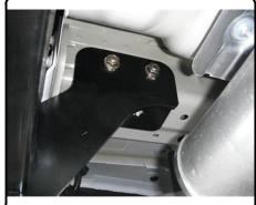
5. Torque all 7/16" fasteners to 59 lb.-ft and all 1/2" fasteners to 110 lb.-ft. Reinstall heat shield and exhaust removed in step 2.
