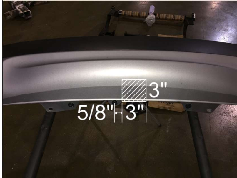
SENSOR BRACKET TRIM DIAGRAM NOTE: REMOVE ANTENNA BEFORE TRIMMING! (IF PRESENT)
