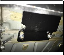
6. Reinstall vehicle exhaust bracket on hitch mounting plate and secure using (2) M10 x 70 and (1) CM-SP1 on each side.
