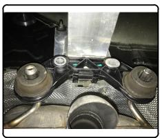
Remove heat shield using needle nose pliers to loosen (4) speed nuts on driver side and (2) speed nuts on passenger. Trim heat shield using aviation shears as shown in Heat Shield Trim Diagram. Reinstall trimmed heat shield.
