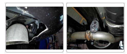
Locate and remove (2) plastic nuts with a 10mm socket. Remove heat shield and mark out a 5" x 13" section with masking tape. Use aviation shears to trim marked area. Reinstall with (1) nut using a 10mm socket.
