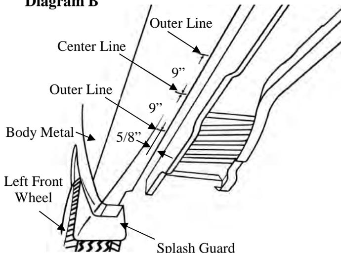
6. Measure 9" from each side of the marked center line on the same body metal surface.
