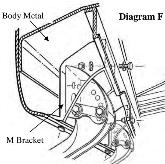
11. Take the remaining 5/16" hardware and bolt the M Brackets to the body metal.
