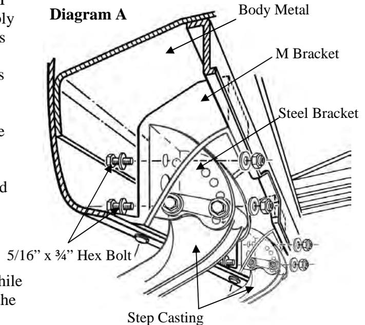
2. Use the 5/16" x 3/4" hex bolts and other 5/16" hardware provided and securely bolt together the steel brackets and M Brackets.
