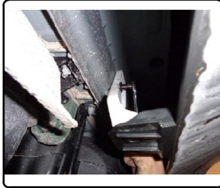
3. Lower the driver side exhaust by removing the rubber isolator from the hanger attached to the vehicle and unbolting the exhaust hanger bracket near the middle of the vehicle using a 13mm socket and ratchet. Repeat on passenger side if present. Support exhaust to prevent damage.
