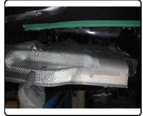
5. BlueTEC vehicles only, temporarily remove (2) bolts holding DEF tank and the (2) nuts securing the strap with an 8mm socket. Support DEF tank to prevent damage.
