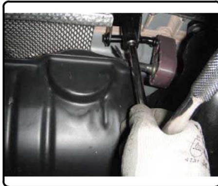
4. Remove the driver side heat shield by removing the (3) formed nuts and (1) bolt with an 8mm socket. Repeat on passenger side if present.
