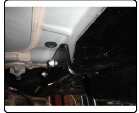
9. Stack bolt plate (D) on spacer plate (E) and run 1/2-13 x 1 1/2" carriage bolts through plate holes. Place plate assembly over the bumper beam tab and align with the holes in the hitch. Secure using 1/2-13 flange nuts, as shown.
