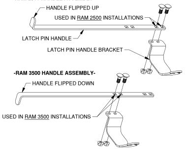
Figure C2: Latch handle assembly configurations.
