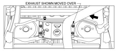
Figure B4: Looking up at frame cross member under truck.
