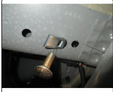
4. Gently pull fascia down and raise hitch into position guiding fishwires through mounting holes. Leave fishwires attached. NOTE: Hardware may need to be temporarily pushed into frame to position hitch over bumper beam studs. Remove fishwires & loosely secure 7/16 nuts. Secure existing M10 nuts onto bumper beam studs.
