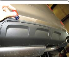
2. Remove (2) screws holding bumper fascia using a T15 torxbit. Save screws for re-installation. Use a 15mm deep well socket to remove (1) M10 flange nut from the bottom of driver side bumper beam attachment location & repeat on passenger side. Save nuts for re-installation.
