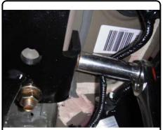
6. Raise exhaust back to original position, and secure exhaust bracket bolts. If present, reattach wire removed in Step (4) to original position.
