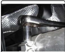
2. On Trailhawk models remove the rear vertical and the horizontal M14 existing bolts from the frame with a 21mm socket, save for reassembly. If wire on passenger side frame rail is present unfasten by pulling the retainer out of the frame, let wire hang below frame rail.
