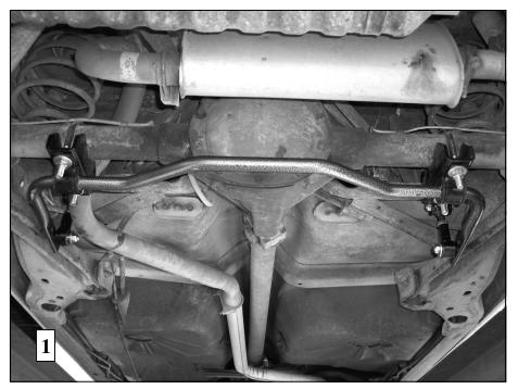
**TORQUE TABLE** Bolt Size 3/8"— 35 ft lbs \* Bolt Size 7/16"— 45 ft lbs \* Bolt Size 1/2"—65 ft lbs \*Bolt Size 9/16"— 90 ft lbs
