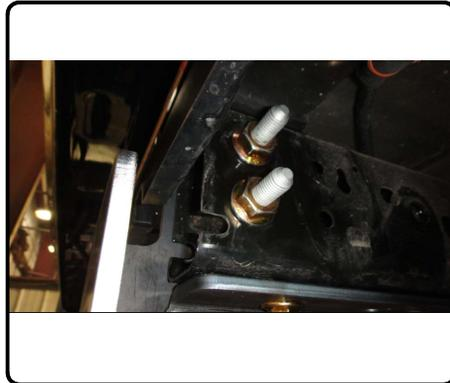
9. Secure the driver side bumper bracket to the hitch using (1) 1/2" hex bolt, (1) conical tooth washer and (1) 1/2" hex flange nut. Repeat on passenger side.
