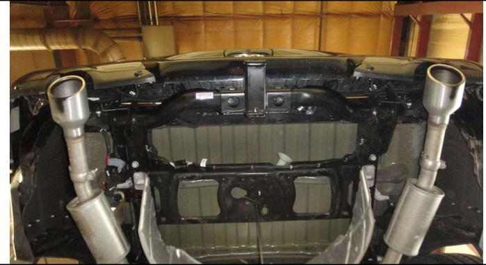
2. On the outside of the driver side frame, unplug the electrical connector. Remove the plastic wiring connectors from the factory hitch.
