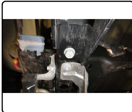
5. Remove (2) factory M6 bolts from the passenger side and (1) M6 bolt on the driver side from the exhaust heat shield. Using a hammer, flatten the heat shield tabs against the frame, heat shield tabs will be pinched between the hitch side plates and the frame.
