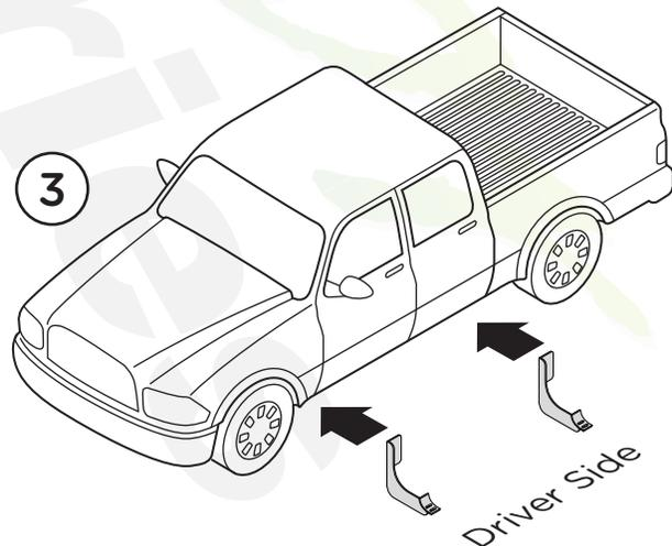
**3.** Install the Driver Side Bolt Plate through the backside of the frame (3a).
