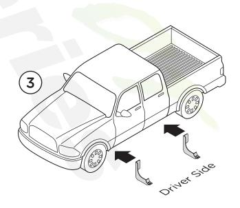
**3.** Install the Driver Side Bolt Plate through the backside of the frame (3a).
